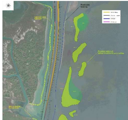
Figure 5 : Detail of the planned morphological structures to the right of the Channel (light green indicates the emerged part - salt marshes - while dark green corresponds to semi-submerged part).
