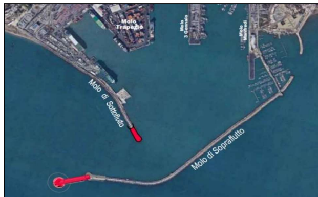
Figure 1. The configuration of the Port of Salerno, red areas indicate the location of the works : the West breakwater was demolished for a length of about 100 m, while the East breakwater has been extended of about 180 m by adopting REWEC3 caissons
